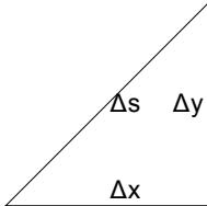
$$\Delta s^2 = \Delta x^2 + \Delta y^2 \Rightarrow \frac{\Delta s^2}{\Delta x^2} = \frac{\Delta x^2 + \Delta y^2}{\Delta x^2} \Rightarrow \frac{\Delta s^2}{\Delta x^2} = 1 + \frac{\Delta y^2}{\Delta x^2} \Rightarrow \frac{\Delta s}{\Delta x} = \sqrt{1 + \frac{\Delta y^2}{\Delta x^2}} \Rightarrow \frac{ds}{dx} = \sqrt{1 + \left(\frac{dy}{dx}\right)^2}$$
